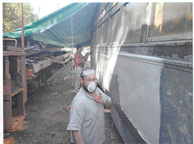
Stripping and Priming on New Jersey Transit car 15
